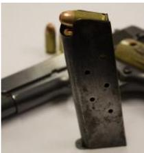
commonly called, holds a several cartridges by their rims and the clip is fed into a magazine leaving the rounds in the magazine. Once the user presses the rounds held in the clip off the strip and down into the magazine—stripping the rounds from the clip, thus the name—the clip is removed. A magazine, in contrast, holds the *entire* cartridge.
